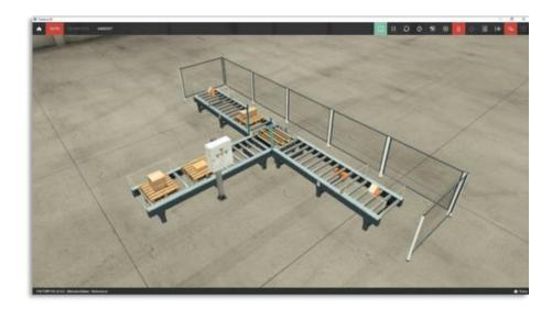
The structuring of the plant is carried out according to Selmo's principles, whereby the stations and processes are divided into logical units (hardware zones and sequences).
