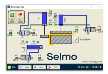
The structuring of the plant is carried out according to Selmo's principles, whereby the stations and processes are divided into logical units (hardware zones and sequences).
