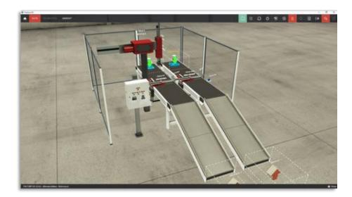
The structuring of the plant is carried out according to Selmo's principles, whereby the stations and processes are divided into logical units (hardware zones and sequences).
